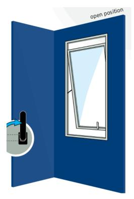
Awning windows open out. Window Handle points upward in open position and at 90° In closed position. Locks at upto 3 points
