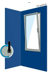
In the Tilt position the handle is Pointing upwards, this position is a secure position whilst letting Ventilation in.
