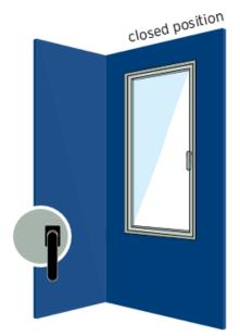
With the Handle Pointing Down The Window is in full lock Position
