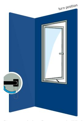
Casement window Case outwards. Window Handle points at 90° in open position and downwards in closed position.
