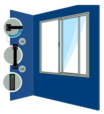
Handle pointing Downwards is lock position and handle at  $90^{\circ}$  is open Position. Keylock handles provided to inactive the handle upon locking with the key. Lockable with upto 3 locking points Maintenance as per notes above
